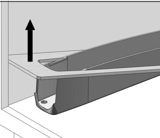
5. Install the Vroom in the mounting bracket by pushing it into place as shown. It will snap in place when installed correctly.
