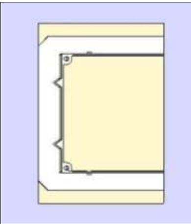
◀ **Insert the rough-in frame** sideways, then turn it back upright behind the wall.
