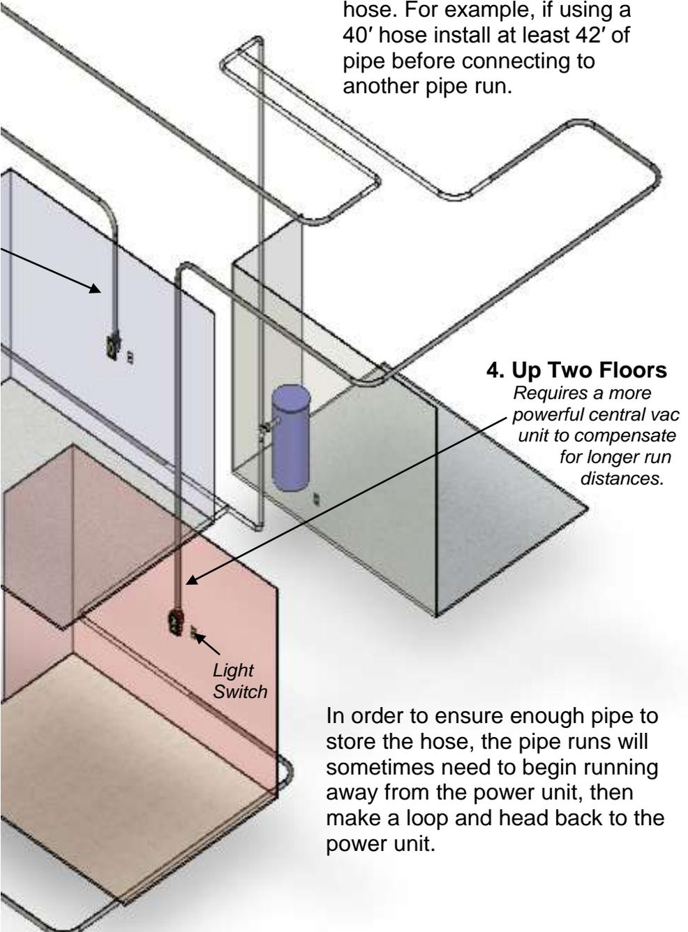
In order to ensure enough pipe to store the hose, the pipe runs will sometimes need to begin running away from the power unit, then make a loop and head back to the power unit.
