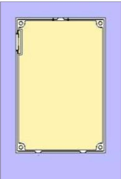
◀ Push the bottom two pointed tabs into the sheet rock. The top pointed tab can be bent down as you pull the top of the frame into the hole. The tabs will help hold the frame into place while you install the valve. You may need to push a couple of small finish nails horizontally into the holes located on the side of the frame.
