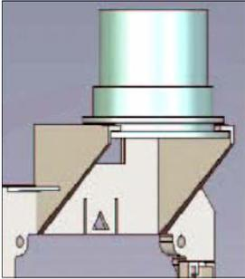
**NOTE:** Valves can be used with a maximum wall thickness of  $\frac{3}{4}$ ". Thicker walls may require modification.
