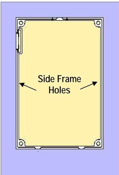
◀ Push the bottom two pointed tabs into the sheet rock. The top pointed tab can be bent down as you pull the top of the frame into the hole. The tabs will help hold the frame into place while you install the valve. You may need to use small finish nails horizontally on the side of the frame to secure the mounting bracket until the valve is installed.
